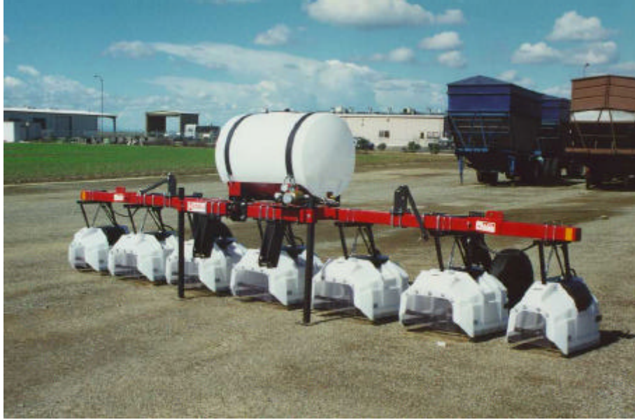
Figure 4. 6-Row, 40" System. The hoods, tank, pump, and hoses are mounted on a tool bar.
